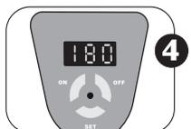
When the unit is plugged in, the display will show the **180** second (3 minute) setting. If a different time is required, press the SET button to cycle the time through the five settings 180s - 280s - 380s - 480s - 90s. Move to the next step when the display shows your required time.
