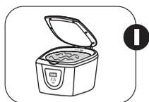
Open the lid and fill the stainless steel tank with warm water (ideally 45 to 50°C). Do not exceed the "MAX" marking on the inside of the tank.
