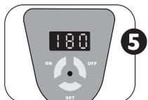
Press the ON button to start cleaning. The red operation indicator will illuminate while the unit is in operation. The built in timer will count down the time automatically.
