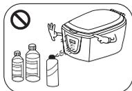
Do not fill the tank with abrasives or corrosive chemicals. Never use acids, solvents or alcohol as these are not suitable for use in this cleaner and will invalidate the warranty. Repeated cleaning cycles will enhance the cleaning effect.
